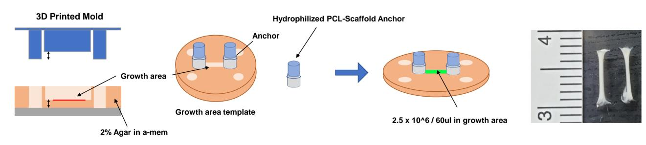
The base of the 3D tendon cell culture was consisted growth area with 2% agaroses with 3D-printed-mold and hydrophilized PCL-scaffold anchors. 3D tendon cell structure was generated tendon cells at 2.5 x 10<sup>6</sup> in the fibronectin-coated growth area between PCL-scaffold anchor. The length of the 3D tendon structure is 7 to 8 mm and the thickness is 0.5 to 1 mm.
